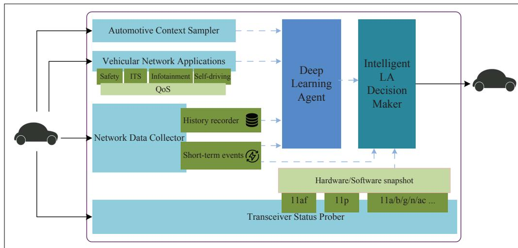
FIGURE 2. Data-driven intelligent LA architecture in 802.11 V2X.
