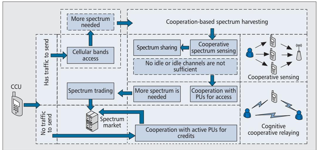
Figure 3. An integrated cooperative framework for spectrum harvesting.
