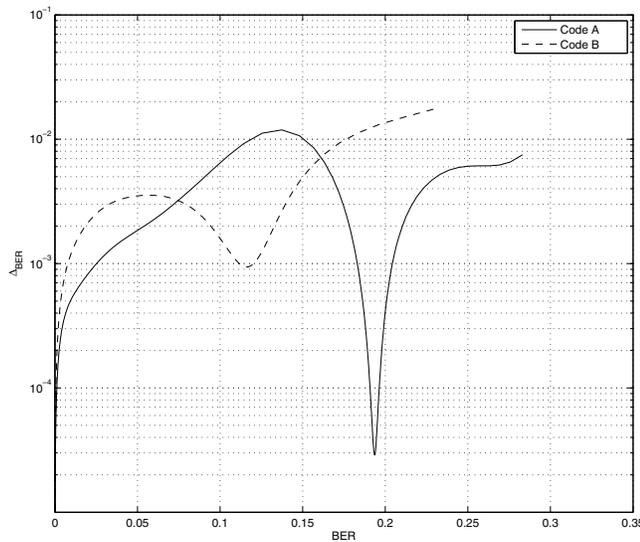
Fig. 10. The decrease of the bit error rate as a function of the current bit error rate.
