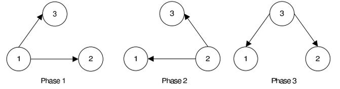
Fig. 1. Three phases in half-duplex two-way relay channels.
