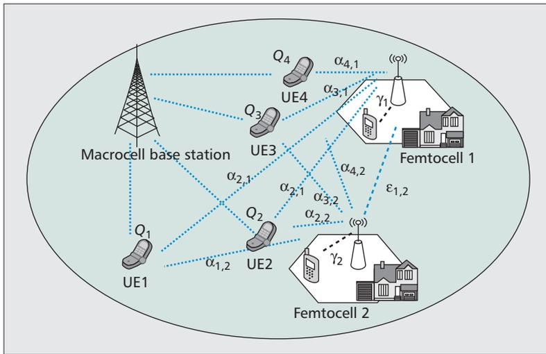
Figure 3. Interference management in cognitive cellular networks.
