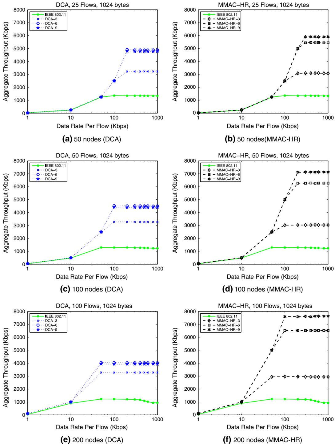
**Figure 4.** The aggregate throughput of the single-hop networks for various numbers of nodes and network loads. The graphs on the left side are the throughput of dynamic channel assignment (DCA), and the graphs on the right side are the throughput of multichannel medium access control protocol with hopping reservation (MMAC-HR).
