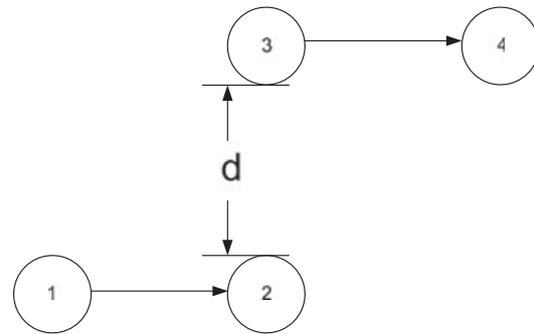
(a) Scenario 1: node 1 transmits to node 2 and node 3 transmits to node 4
