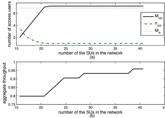
Fig. 11. Relation between the number of the SUs in the network,  $M_{B2}$ , and: (a) the average number of the RT access users,  $\bar{M}_{rt}$ , NRT access users,  $\bar{M}_{nrt}$ , and NRT allocated channels,  $\bar{n}_{nrt}$ , and (b) the network average aggregate throughput,  $\bar{O}$ ; for  $N = 20$  channels,  $\delta = 0.3$ ,  $P_D = 0.01$ ,  $P_B = 0.1$ , and  $l = 20$  packets.
