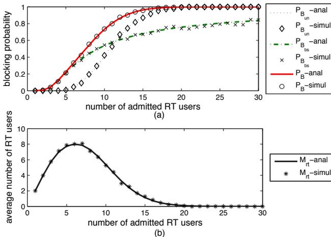
Fig. 5. Relation between the number of the admitted RT users,  $A_{rt}$ , and (a) blocking probabilities,  $P_B$ ,  $P_{B_{un}}$ ,  $P_{B_{bs}}$  and (b) average number of the RT users in the network,  $\bar{M}_{rt}$ ; for  $N = 20$  channels,  $\delta = 0.3$ ,  $P_D = 0.01$ , and  $l = 20$  packets.
