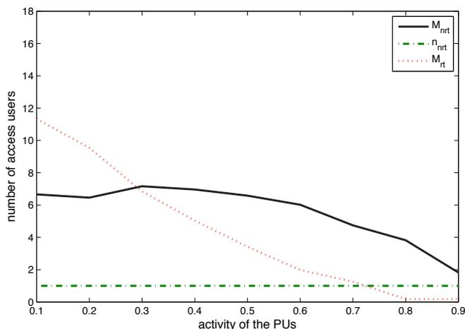
Fig. 14. Average number of the RT access users,  $\bar{M}_{rt}$ , NRT access users,  $\bar{M}_{nrt}$ , and NRT allocated channels,  $\bar{n}_{nrt}$ , for different values of the activity of the PUs,  $\delta$ ; for  $N = 20$  channels,  $P_D = 0.01$ ,  $P_B = 0.1$ , and  $l = 20$  packets.
