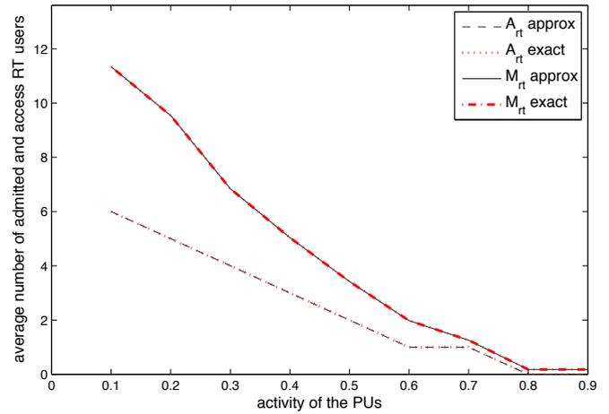
Fig. 9. Approximated and exact number of admitted RT users,  $A_{rt}$ , and access RT users,  $\overline{M}_{rt}$ , for different values of the activity of the PUs,  $\delta$ ; for  $N = 20$  channels,  $P_D = 0.01$ ,  $P_B = 0.1$ , and  $l = 20$  packets.
