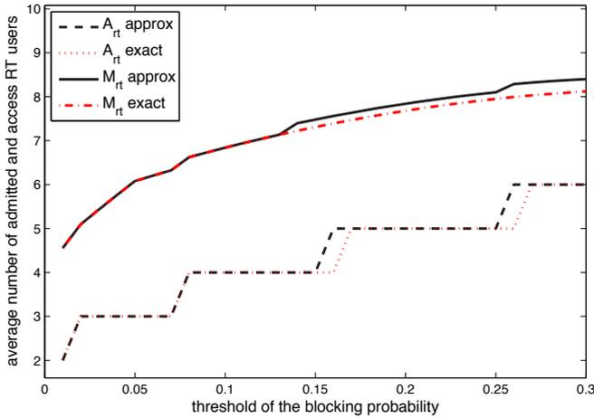
Fig. 7. Approximated and exact number of admitted RT users,  $A_{rt}$ , and access RT users,  $\overline{M}_{rt}$ , for different threshold values of the blocking probability,  $P_B$ ; for  $N = 20$  channels,  $\delta = 0.3$ ,  $P_D = 0.01$ , and  $l = 20$  packets.
