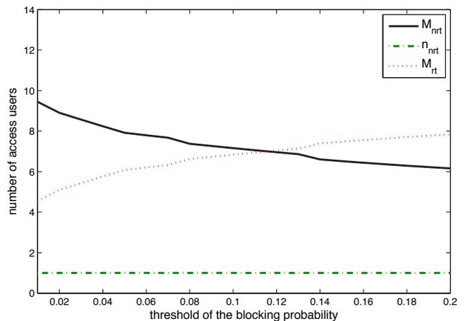
Fig. 13. Average number of the RT access users,  $\bar{M}_{rt}$ , NRT access users,  $\bar{M}_{nrt}$ , and NRT allocated channels,  $\bar{n}_{nrt}$ , for different threshold values of the blocking probability,  $P_B$ ; for  $N = 20$  channels,  $\delta = 0.3$ ,  $P_D = 0.01$ , and  $l = 20$  packets.
