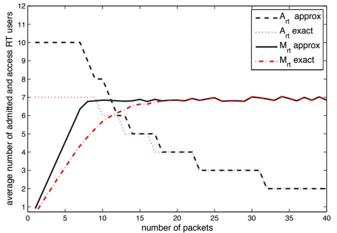
Fig. 6. Approximated and exact number of admitted RT users,  $A_{rt}$ , and access RT users,  $\bar{M}_{rt}$ , for different number of packets,  $l$ , when  $N = 20$  channels,  $\delta = 0.3$ ,  $P_D = 0.01$ , and  $P_B = 0.1$ .
