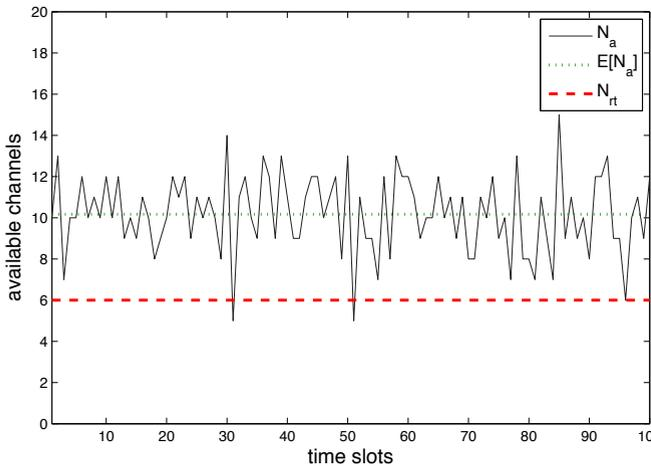
Fig. 4. Simulation of the available channels,  $N_a$ , their mean,  $E[N_a]$ , and the number of the channels that can support RT users,  $N_{rt}$ ; for  $N = 20$  channels,  $\delta = 0.5$ , and  $P_D = 0.01$ .
