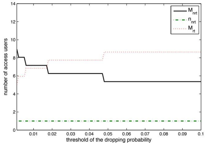
Fig. 12. Average number of the RT access users,  $\bar{M}_{rt}$ , NRT access users,  $\bar{M}_{nrt}$ , and NRT allocated channels,  $\bar{n}_{nrt}$ , for different threshold values of the dropping probability,  $P_D$ ; for  $N = 20$  channels,  $\delta = 0.3$ ,  $P_B = 0.1$ , and  $l = 20$  packets.
