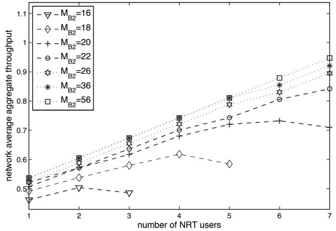
Fig. 10. The network aggregate throughput,  $\Theta$ , with respect to the number of the NRT access users,  $M_{nrt}$ , for different numbers of the users in the network,  $M_{B2}$ ; for  $N = 20$  channels,  $\delta = 0.3$ ,  $P_D = 0.01$ ,  $P_B = 0.1$ , and  $l = 20$  packets.
