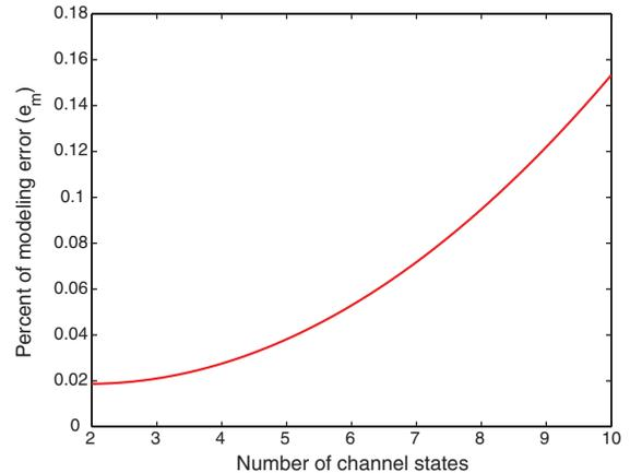
Fig. 4. Modeling error for the channel of a single versus the resolution of the Markov model (number of states).
