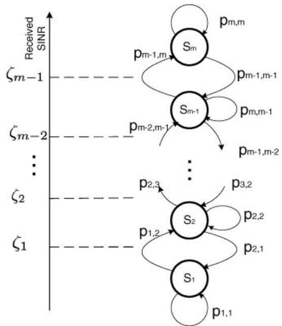
Fig. 12. Finite-state Markov model for fading channels.
