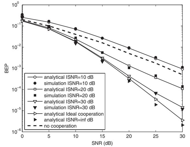
Fig. 6. Bit error probability of the CD system with 16-QAM for similar channel towards BS.
