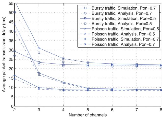
Fig. 6. TS: delay vs. number of channels.
