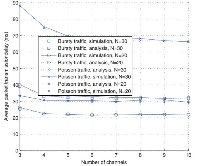
Fig. 4. PS: delay vs. number of channels.
