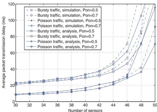
Fig. 7. TS: delay vs. number of sensors.
