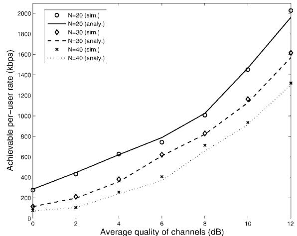
Fig. 12. Achievable per-user rate versus the average quality of wireless channels for an unsaturated case.
