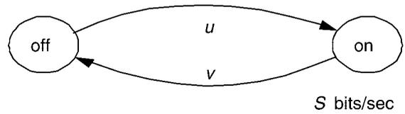
Fig. 10. On-off traffic source model.
