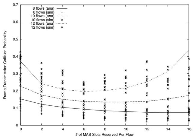
Fig. 7. Frame collision probability: simulation and analysis results.
