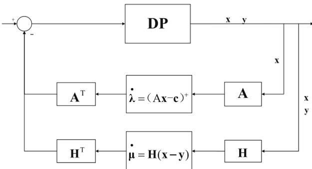
Fig. 1. Close-loop system framework of algorithm DAULT.
