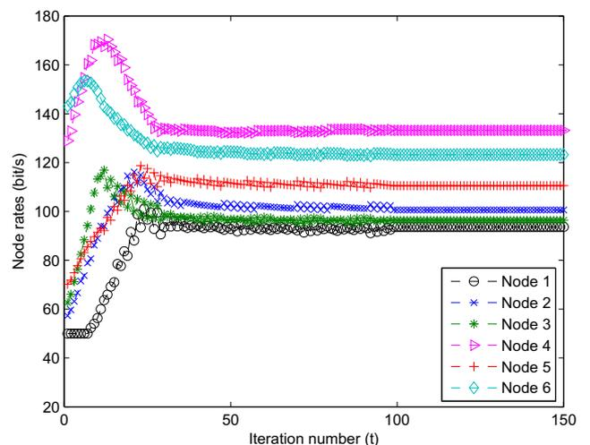
Fig. 4. The convergent performance of the *Algorithm DAULT*,  $\gamma = 0.95$ .
