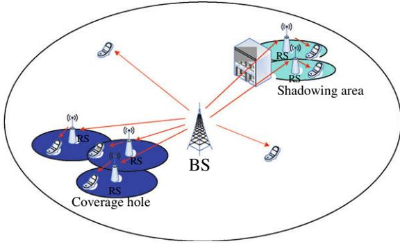
Fig. 3. The typical topology of relay network.
