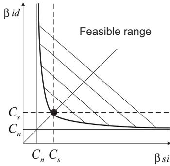
Fig. 2. Range of channel gains for the feasibility of relay nodes.
