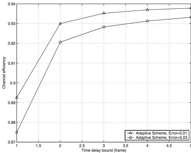
Fig. 10. Channel efficiency for the ADP scheme.
