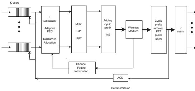
Fig. 1. Real-time video transmission over OFDM wireless channels.
