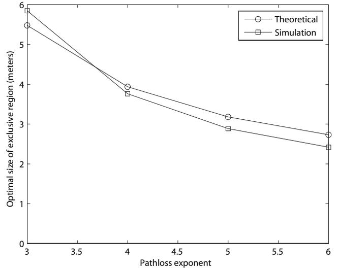
Fig. 3. Optimal radius of exclusive region with the following parameters in Eq. (7):  $p_t = 0.05$  mW,  $N_0 = 2.5 \times 10^{-8}$  mW, and  $bk = 10^{-4}$ .
