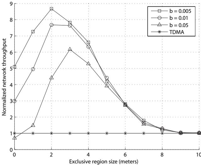
Fig. 8. Normalized network throughput due to different MUI factor  $b$  with 40 flows in  $10 \times 10 \text{ m}^2$ , Nakagami- $m=4$ . In this setting the optimal exclusive size is between  $2 \sim 4 \text{ m}$ .
