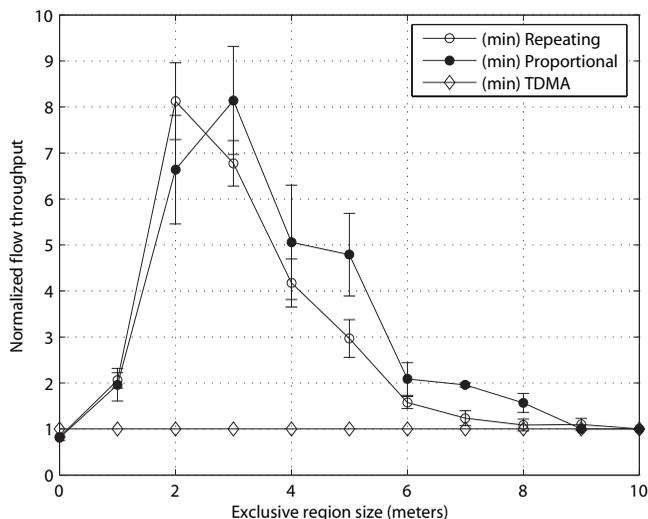
Fig. 7. The minimum flow rate achieved by each algorithm. with 40 flows in  $10 \times 10 \text{ m}^2$ ; Nakagami- $m=4$ ; MUI factor  $b=10^{-2}$ . The error bars represent 95% confidence interval.
