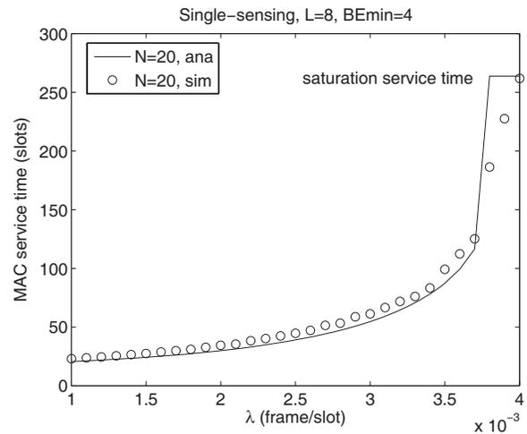
Fig. 9. Average frame service time in unsaturated case
