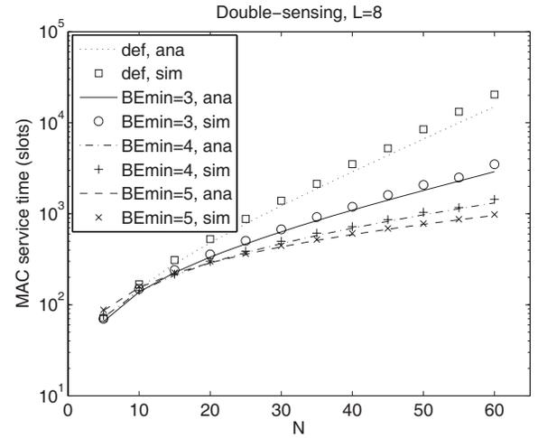
Fig. 4. Average frame service time in saturated case
