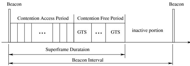
Fig. 1. IEEE 802.15.4 superframe structure in the beacon-enabled mode
