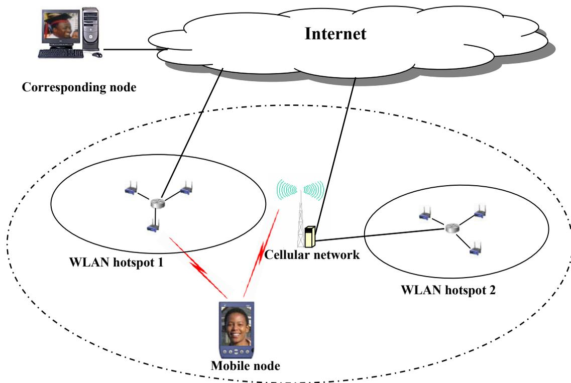
Fig. 1. An integrated WLAN and cellular networks architecture.
