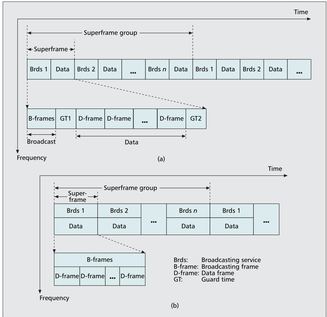
■ Figure 2. Superframe structure of a) TDM; b) FDM.
