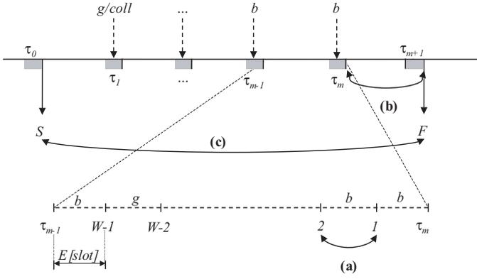
Fig. 2. Transmission success/failure behaviors in the IEEE 802.11 WLANs: (a) a slot, (b) a backoff stage, (c) a packet transmission interval. *coll*, *S*, and *F* represent collision, successful transmission, and failed transmission, respectively.
