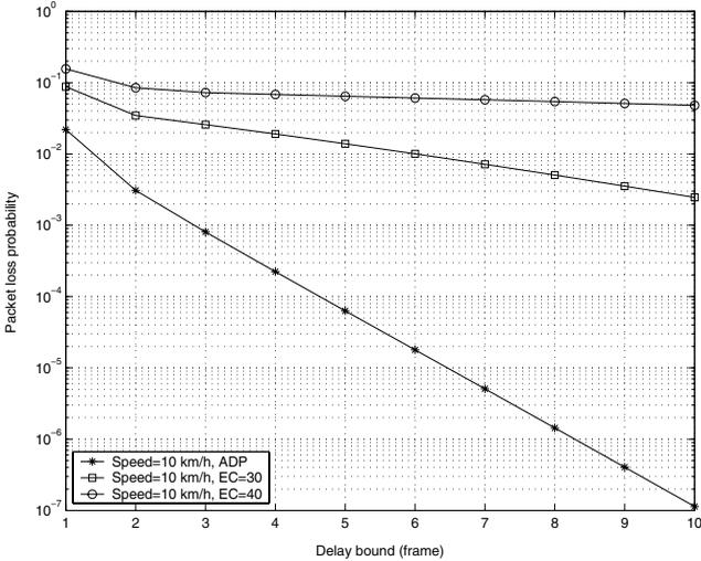
Fig. 9. Comparison of packet loss probabilities for Rate-adaptation and EC schemes.
