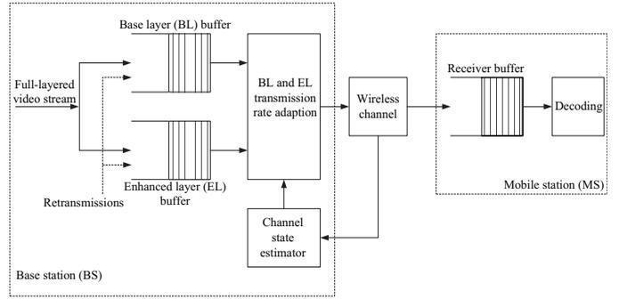
Fig. 1. Adaptive multi-layered video transmission over the wireless medium.
