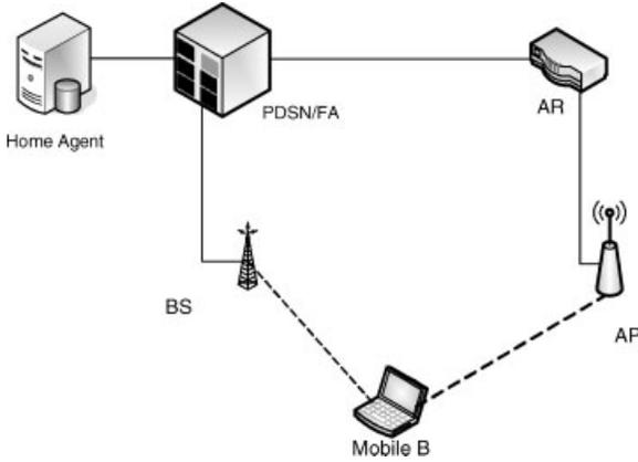
Fig. 7. Simplified network model for vertical handoff.
