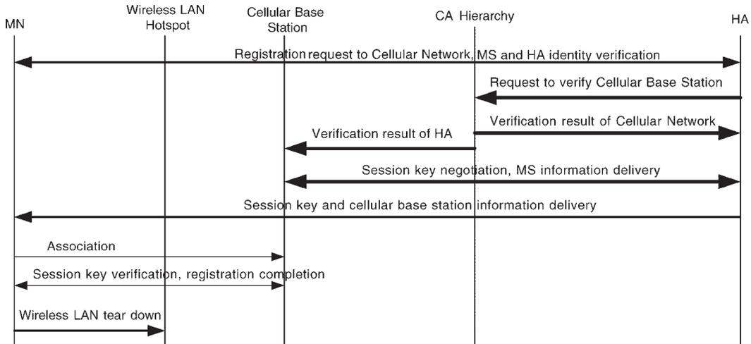
Fig. 4. Upward registration signaling.
