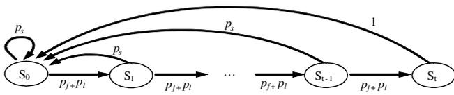
Fig. 11. State transition diagram of each member node.
