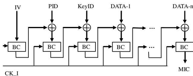
Fig. 9. Message integrity check mechanisms (BC: Block Cipher).
