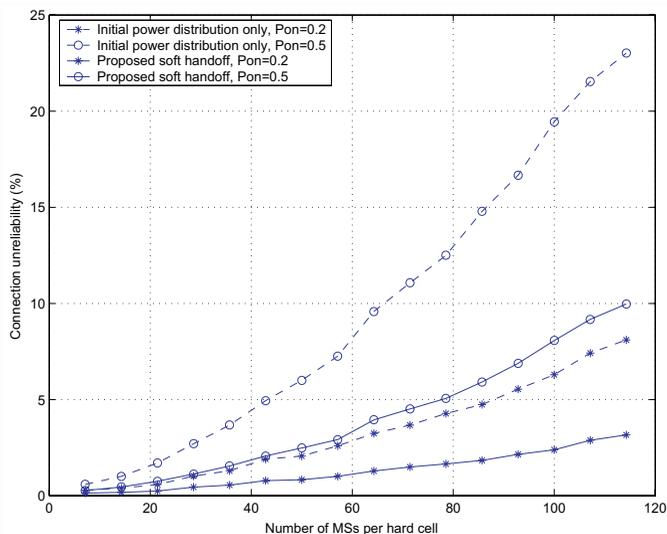
Fig. 6. Comparison between the proposed SHO scheme and the scheme with initial power allocation only.
