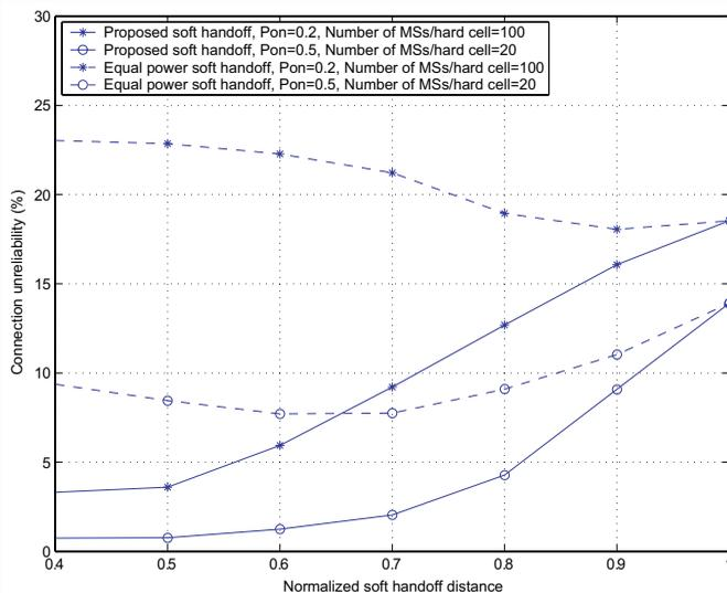
Fig. 7. Comparison between the proposed SHO scheme and the equal power soft handoff scheme.
