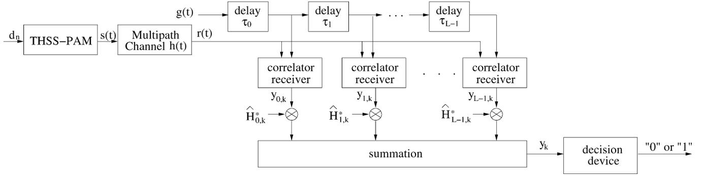
Fig. 1. Transceiver structure of the UWB system.
