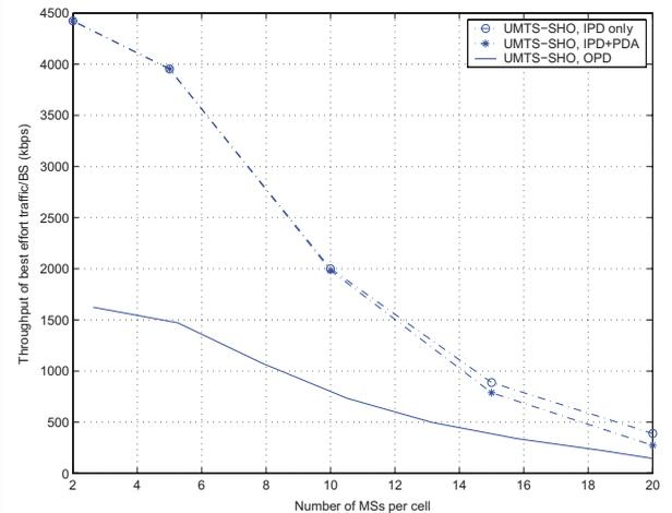
Fig. 7. Throughput of best effort traffic using the UMTS-SHO scheme
