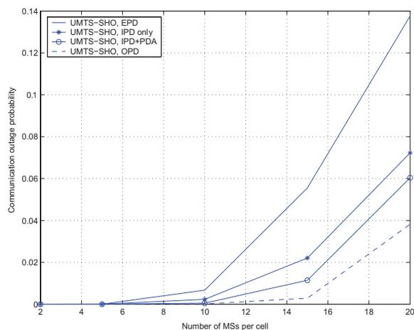
Fig. 3. Outage probability using the UMTS-SHO scheme
