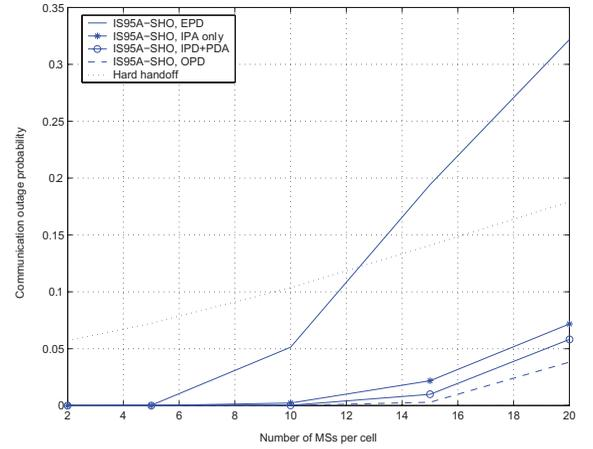
Fig. 1. Outage probability using the IS95A-SHO scheme
