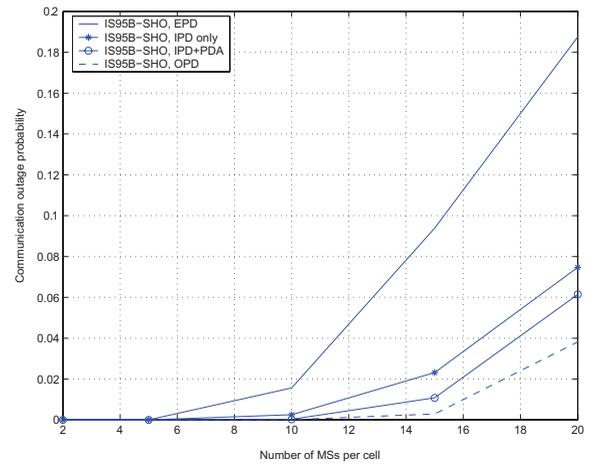
Fig. 2. Outage probability using the IS95B-SHO scheme
