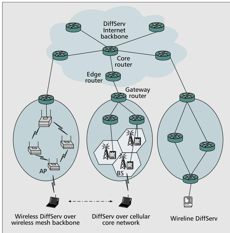
■ Figure 2. A DiffServ platform for network interconnection.
