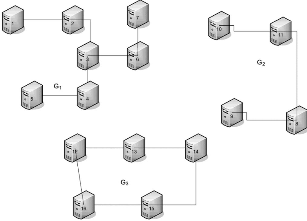
Fig. 7. Three wireless access networks with partial mesh topology.
