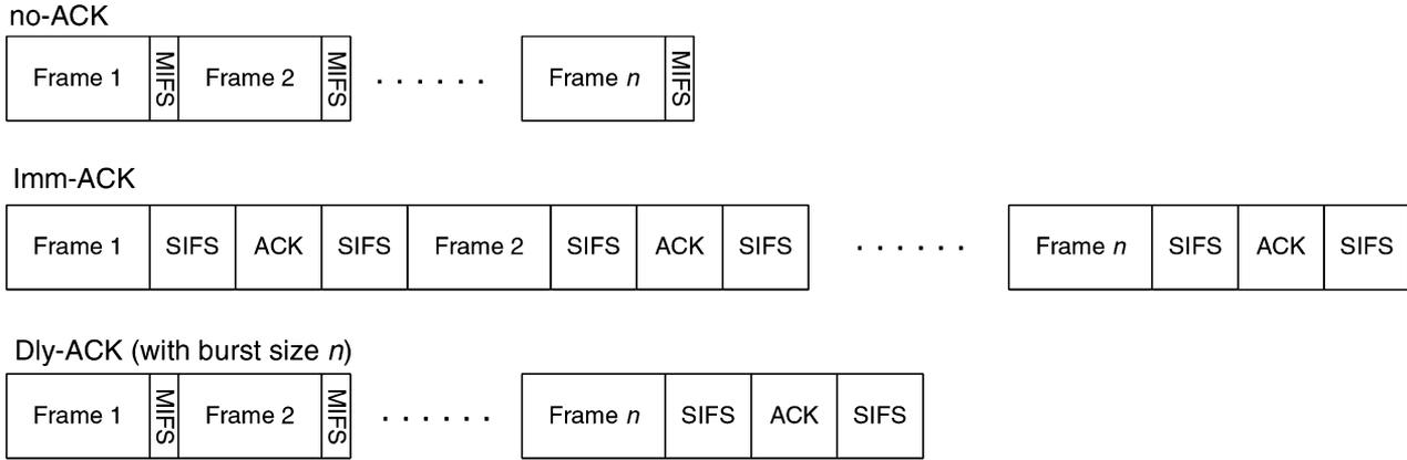
Fig. 7. No-ACK, Imm-ACK, and Dly-ACK mechanisms in IEEE 802.15.3.
