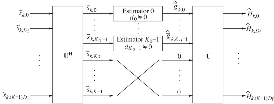
Fig. 5. Joint time–frequency channel estimator for OFDM system.
