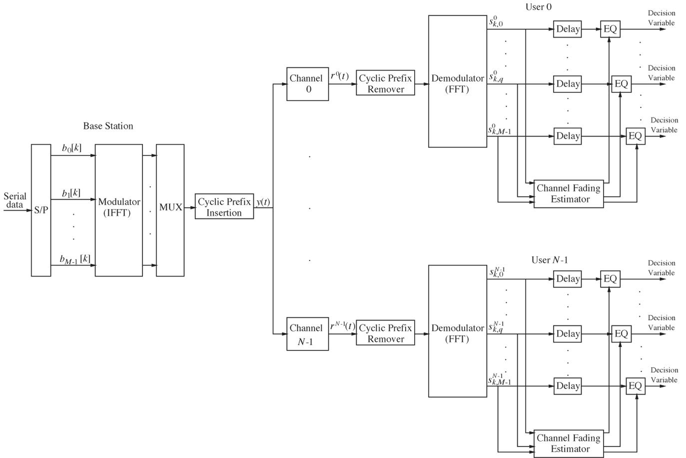
Fig. 1. Transceiver structure of the OFDM system.
