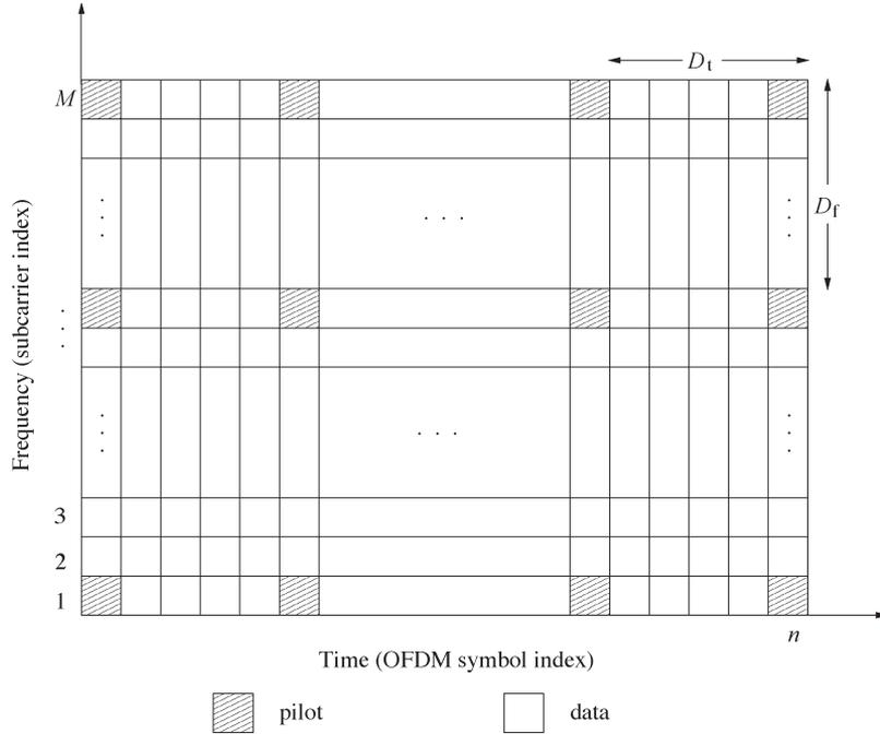
Fig. 4. Configuration of pilot arrangement.
