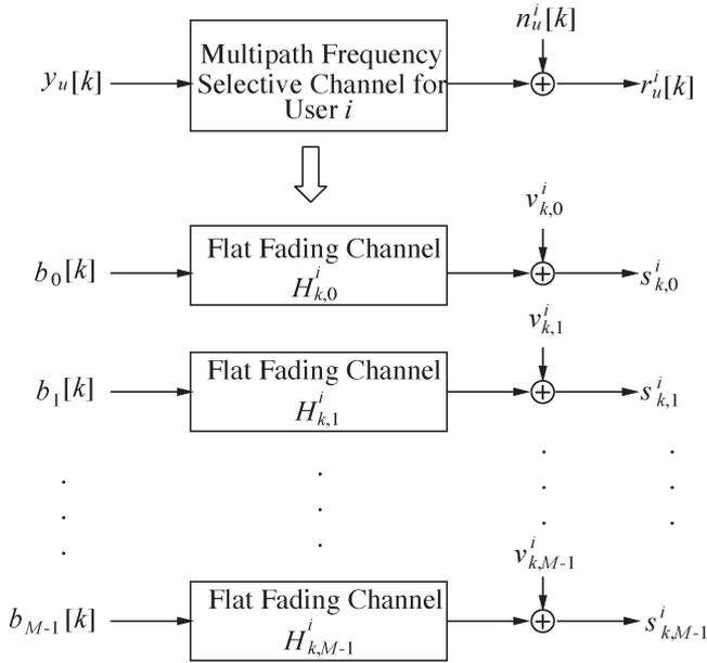
Fig. 2. Equivalent channel model for user  $i$ .
