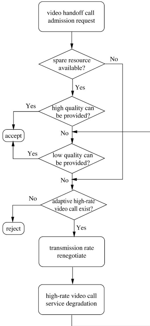
Fig. 5. Video handoff call admission control diagram.
