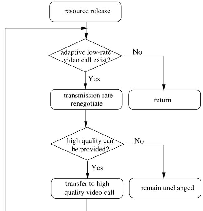
Fig. 6. Low-quality video call transmission rate adjustment.
