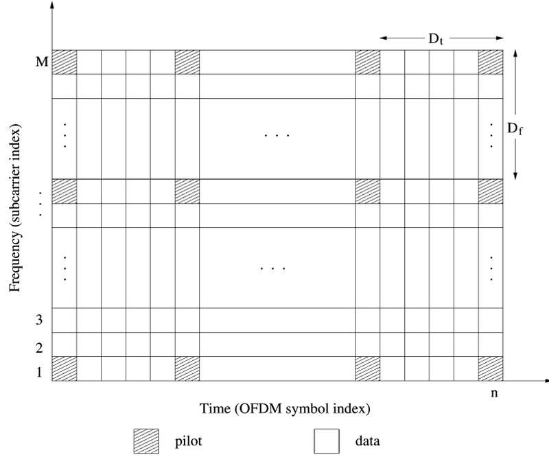
Fig. 2. Configuration of pilot arrangement.
