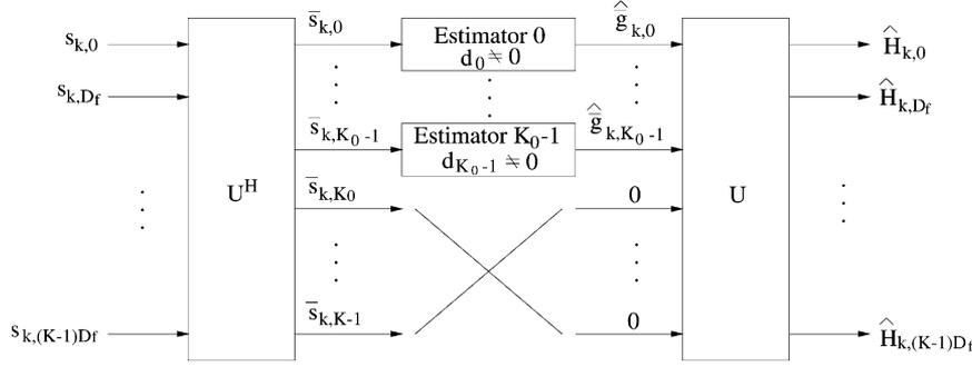
Fig. 3. Joint time–frequency channel estimator for OFDM system.
