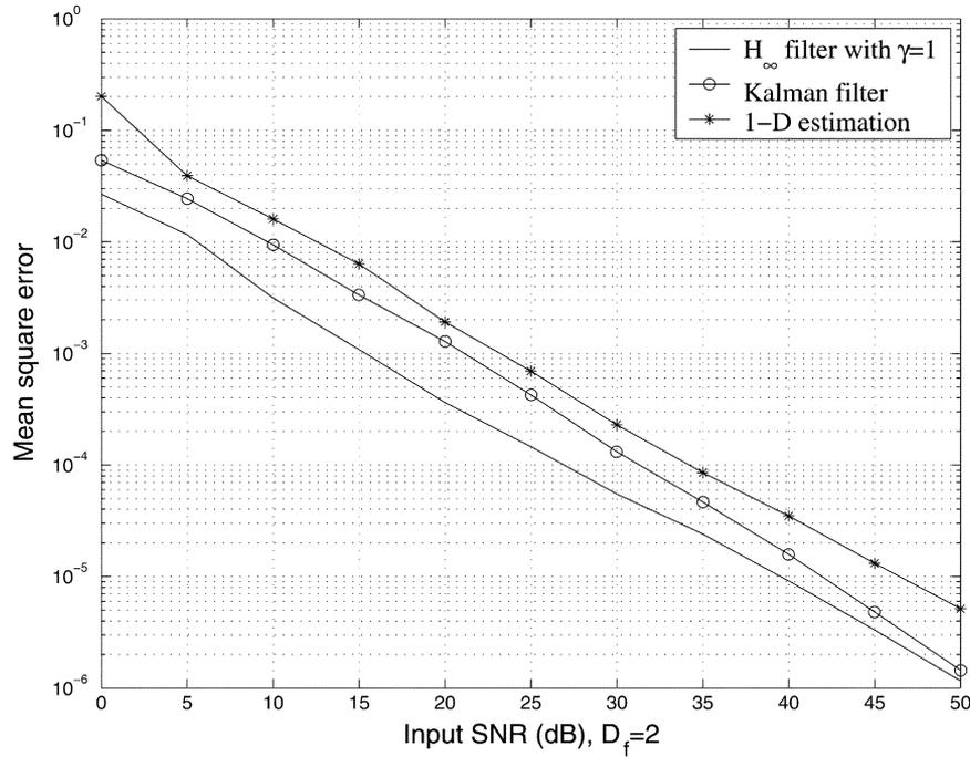
Fig. 5. Mean-square-error performance over different input SNR.
