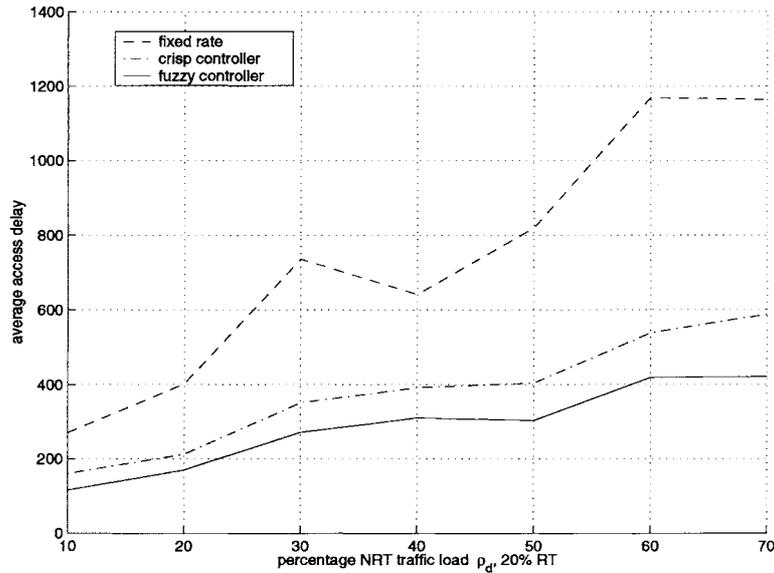
Figure 9. Effect of increasing  $\rho_d$  with  $\%RT = 20$ ;  $\kappa = 2.7$ .
