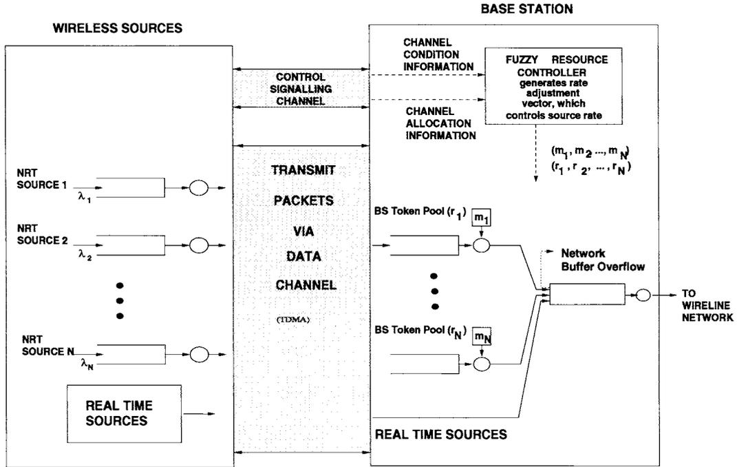
Figure 1. System model of the fuzzy resource allocator.
