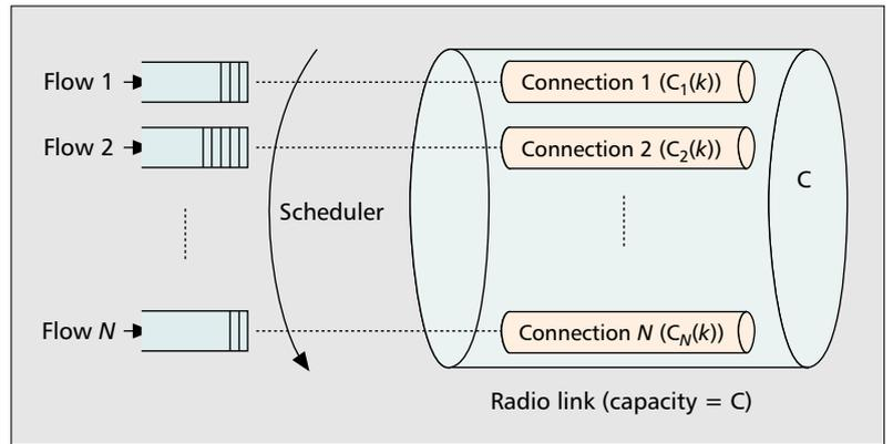
Figure 4. A queuing model of the CDGPS scheme.
