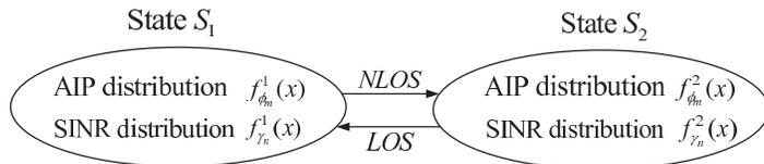
Fig. 2: Non-stationary channel model with two states.
