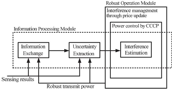
Fig. 3: System structure for robust power control
