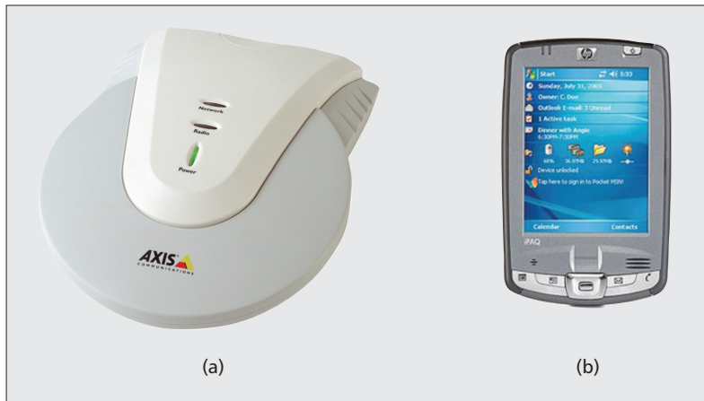
Figure 3. Main equipment for the experiment in our feasibility study: a) an AXIS 9010 Bluetooth™ AP; b) an HP iPAQ hx2790c Pocket PC.
