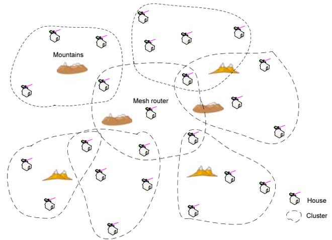
Fig. 1. An illustration of a clustered WMN, where stationary wireless routers are mounted on rooftops of a residential area.
