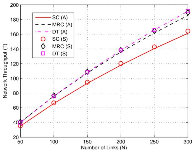
(b)  $\omega = \pi/3$  and  $\lambda_R = 0.0002$  nodes/m<sup>2</sup>Fig. 10: Network throughput versus total number of links when  $d_{SD} = 50$  m.
