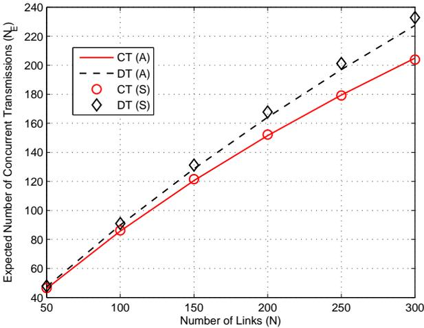
Fig. 8: Expected numbers of concurrent direct and cooperative transmissions versus total number of links when  $\omega = \pi/3$ ,  $\lambda_R = 0.003$  nodes/m<sup>2</sup>, and  $d_{SD} = 50$  m.
