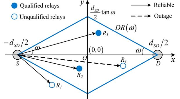
Fig. 2: A diamond-shaped constrained relay selection region under the rectangular coordinate system. Only the relays within the constrained relay selection region (e.g.,  $R_2, R_3$ , and  $R_4$ ) and successfully receive the packet from the source (e.g.,  $R_2$  and  $R_3$ ) are qualified relays (e.g.,  $R_2$  and  $R_3$ ).
