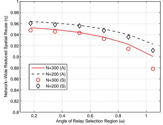
Fig. 9: Network-wide reduced spatial frequency reuse versus angle of relay selection region for  $N = 200$  and 300 when  $\lambda_R = 0.003$  nodes/m<sup>2</sup> and  $d_{SD} = 50$  m.
