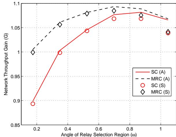
Fig. 11: Network throughput gain versus angle of relay selection region when  $\lambda_R = 0.003$  nodes/m<sup>2</sup>,  $d_{SD} = 50$  m, and  $N = 300$ .
