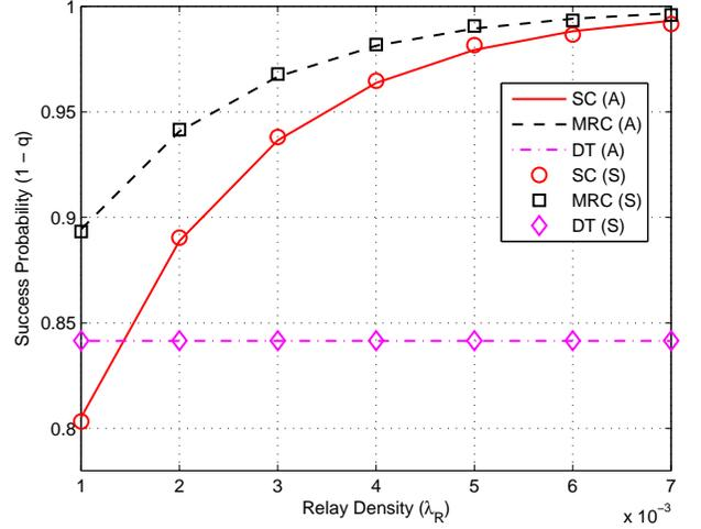
Fig. 6: Success probability versus relay density (in nodes/m<sup>2</sup>) when  $\omega = \pi/6$  and  $d_{SD} = 50$  m.
