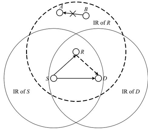
Fig. 1: IR enlargement due to relay transmission under the protocol interference model.
