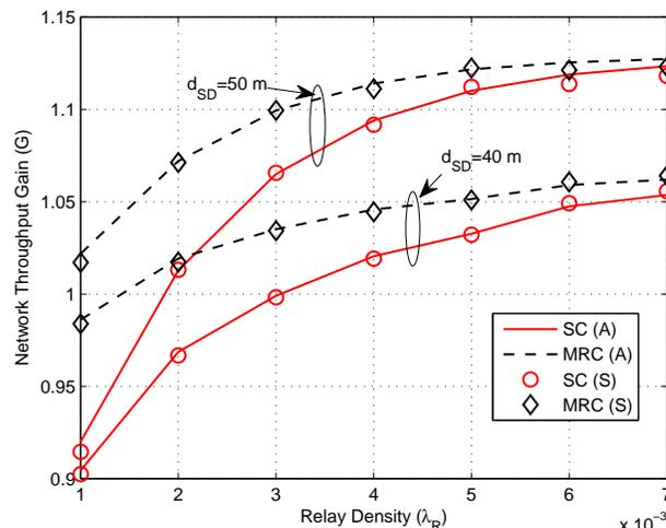
Fig. 12: Network throughput gain versus relay density (in nodes/m<sup>2</sup>) for  $d_{SD} = 40$  m and 50 m when  $\omega = \pi/6$  and  $N = 200$ .
