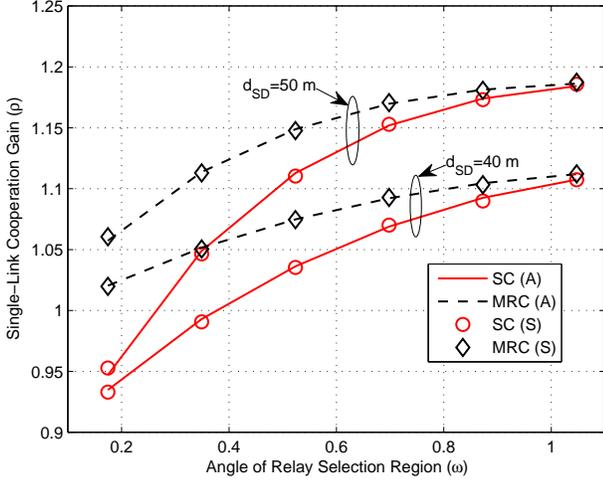
Fig. 7: Single-link cooperation gain versus angle of relay selection region for  $d_{SD} = 50$  m and 40 m when  $\lambda_R = 0.003$  nodes/m<sup>2</sup>.
