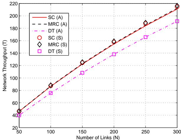
(a)  $\omega = \pi/6$  and  $\lambda_R = 0.006$  nodes/m<sup>2</sup>
