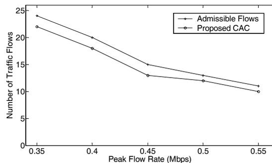
Fig. 3. Admitted flows from the proposed scheme and admissible flows with different flow rates.
