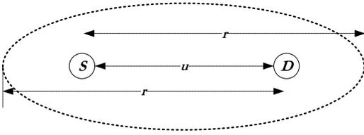
Fig. 4. Illustration of the common coverage road segment of an  $s-d$  pair.
