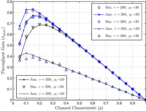
Fig. 10. Throughput gain of CAH MAC over ADHOC MAC with  $F = 60$  time slots.
