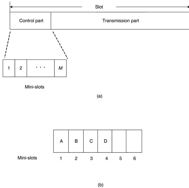
Fig. 2. The slot structure in the proposed scheme.
