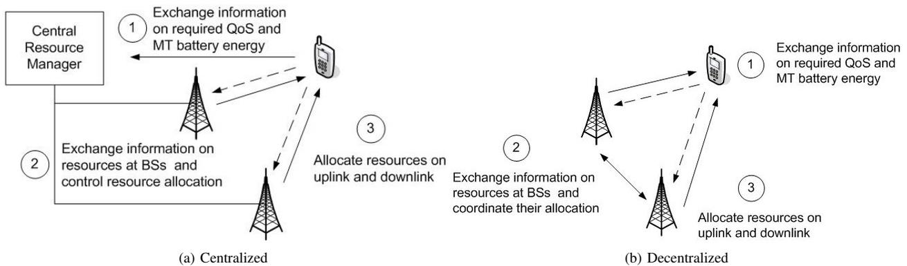
Fig. 3. Centralized and decentralized implementations.
