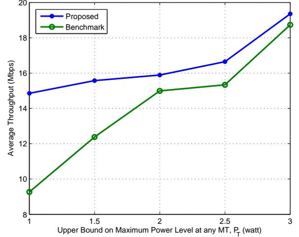
Fig. 5. Throughput versus the upper bound of the maximum power level,  $P_T$ , at any MT [13].
