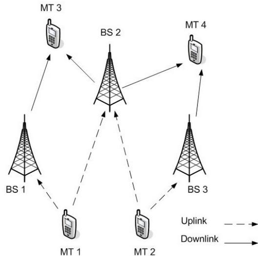
Fig. 2. An illustration of multi-homing uplink and downlink radio communications in a heterogeneous wireless medium.
