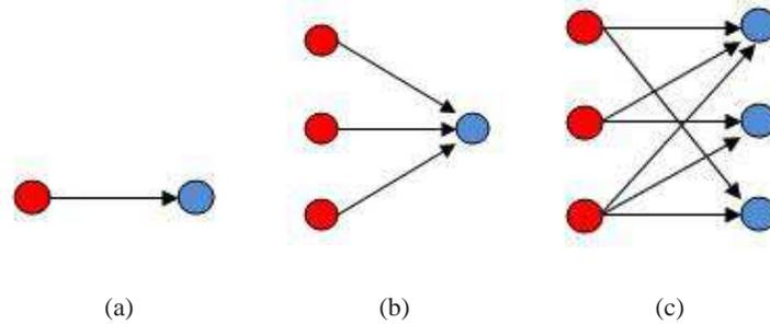
Fig. 4. Link definitions in cooperative networks: (a) Point-to-point; (b) MISO; (c) MIMO.
