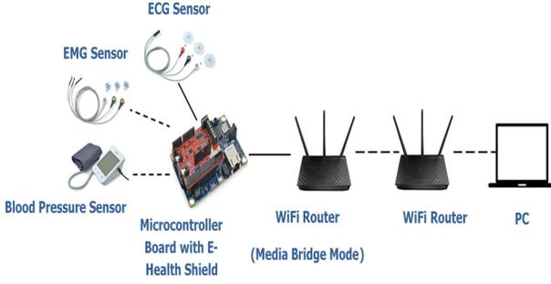
Fig. 2: Experimental setup for e-health data trace.
