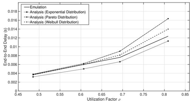
Fig. 15: End-to-end delay from a WiFi gateway to a management server (video surveillance pattern).
