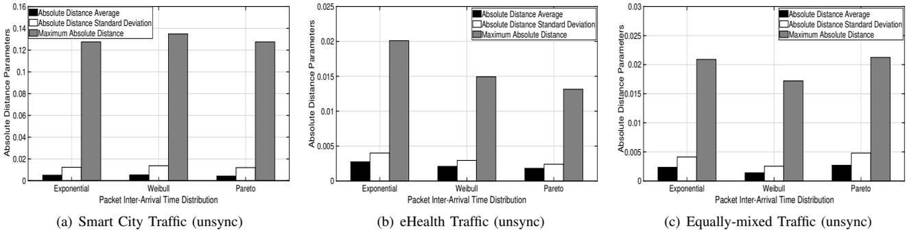
Fig. 12: Absolute distance parameters for the unsynchronized traffic Pattern 2, 3, and 4.
