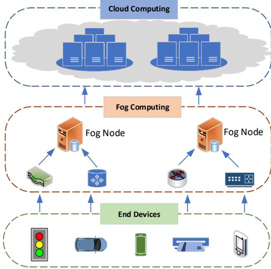
Fig. 1: Fog-to-cloud Data Management Architecture
