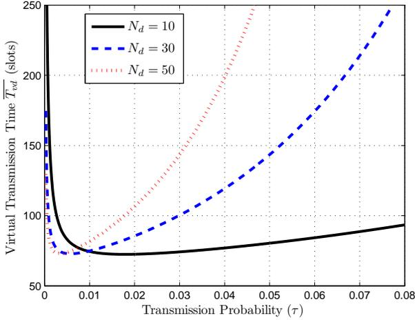
Fig. 5: The evaluation of  $\overline{T}_{vd}$  in a function of  $\tau$  ( $\varphi = 0.5$ ,  $N_v = 20$ ).
