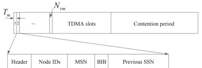
Fig. 2: Format of control packet broadcast in each minislot.
