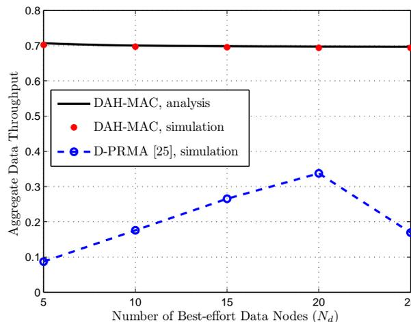
Fig. 14: A comparison of the DAH-MAC maximum data throughput ( $\varphi = 0.33$ ,  $N_v = 10$ ) with the D-PRMA protocol.
