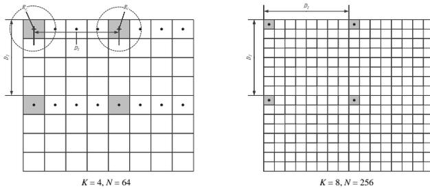
**Fig. 1** An illustration of restricted TDMA MAC under different node density scenarios with  $K = 16$  and  $K = 64$ , respectively. The dots at the center of each cell represent nodes, and grey cells can transmit simultaneously.
