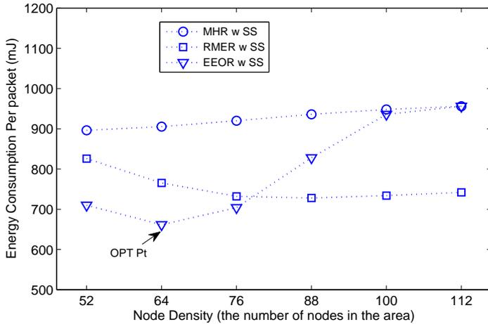
**Fig. 12** Energy consumption per packet versus the node density under the use of routing protocols with sleep scheduling
