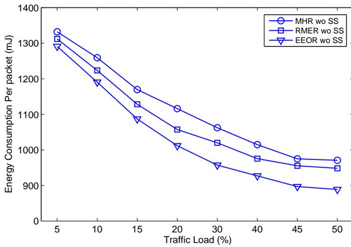
**Fig. 6** Energy consumption per packet versus the traffic load under the use of routing protocols without sleep scheduling
