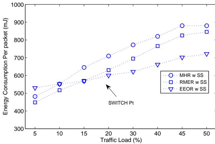
**Fig. 7** Energy consumption per packet versus the traffic load under the use of routing protocols with sleep scheduling
