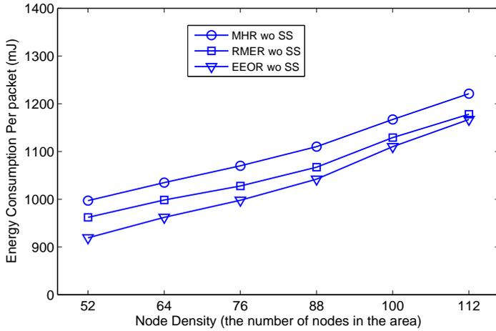
**Fig. 11** Energy consumption per packet versus the node density under the use of routing protocols without sleep scheduling
