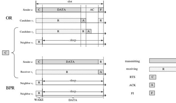
**Fig. 2** An illustration of the routing operation within a single time slot
