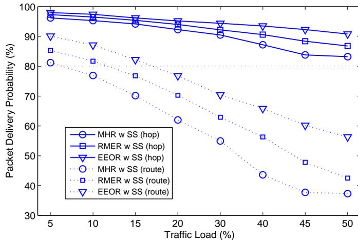
Fig. 3 The packet delivery probability versus the traffic load
