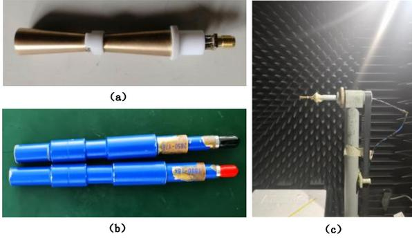
Fig. 9. (a) Photograph of the prototype. (b) A traditional calibration dipole. (c) Measurement set-up in the anechoic chamber.
