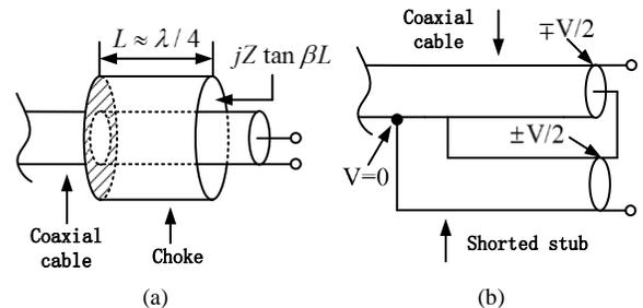
Fig. 1. (a) Current balun. (c) Voltage balun.
