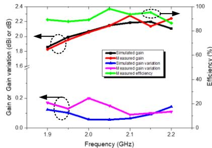
Fig. 12. Simulated and measured gain, gain variation in the horizontal plane and measured efficiency of the proposed dipole.
