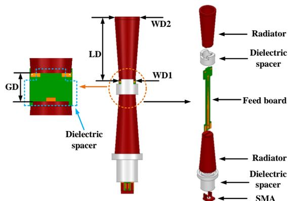
Fig. 2. Antenna structure.
