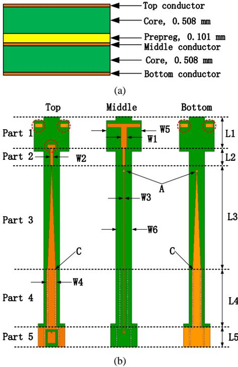
Fig. 3. Structure of the balun and related feeding network. (a) Board stackup. (b) Wiring layout.
