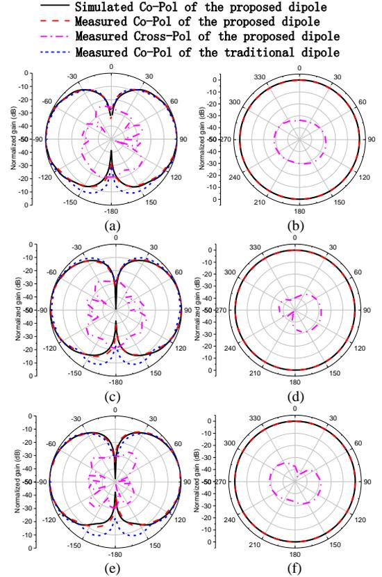
Fig. 11. Simulated and measured patterns of the proposed dipole and measured vertical patterns of a traditional dipole. (a) Vertical plane at 1.9 GHz. (b) Horizontal plane at 1.9 GHz. (c) Vertical plane at 2.05 GHz. (d) Horizontal plane at 2.05 GHz. (e) Vertical plane at 2.2 GHz. (f) Horizontal plane at 2.2 GHz.
