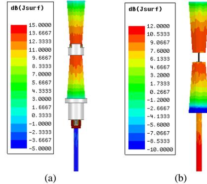
Fig. 7. Simulated current distribution at 2 GHz (a) with and (b) without the designed balun.
