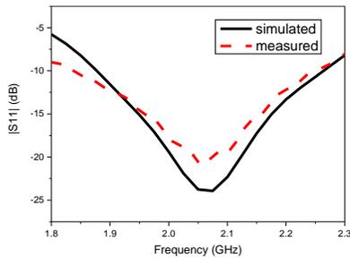
Fig. 10. Simulated and measured  $|S_{11}|$  of the proposed dipole.
