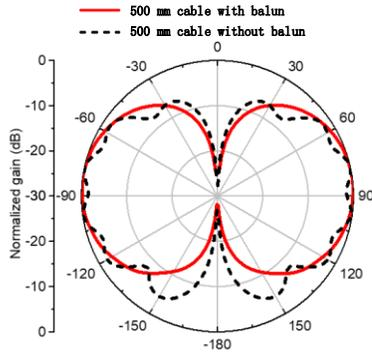
Fig. 8. Simulated vertical radiation patterns with and without the designed balun at 2 GHz.
