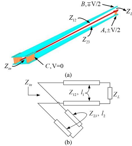
Fig. 5. (a) Working principle of the proposed voltage balun. (b) Equivalent circuit of the proposed voltage balun.
