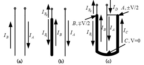
Fig. 4. (a) Balanced transmission line. (b) Unbalanced transmission line. (c) Unbalanced transmission line with a voltage balun.
