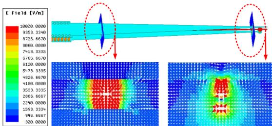
Fig. 6. Electric field distribution in the tapered transmission line.
