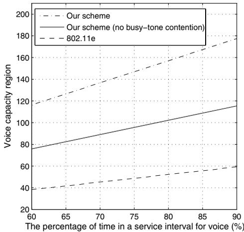
Fig. 12. The analyzed voice traffic capacity region of our proposed scheme, our scheme without busy-tone contention mechanism, and IEEE 802.11e.
