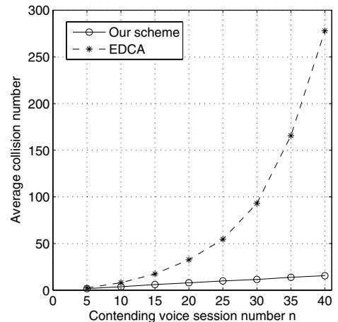
Fig. 7. Average collision number in a CP when our scheme or EDCA is applied with  $CW_{min} = 3$  and  $CW_{max} = 15$ .
