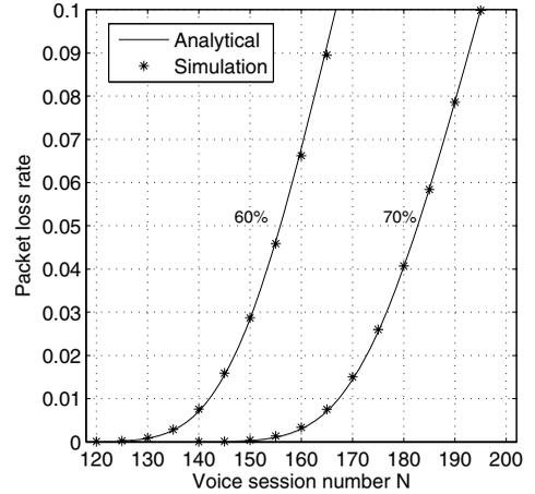
Fig. 10. Packet loss rate in CFP for  $T_{CFP} = 60\%T_{SI}$  and  $T_{CFP} = 70\%T_{SI}$  in our scheme.
