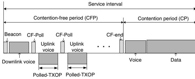
Fig. 2. The structure of a service interval.
