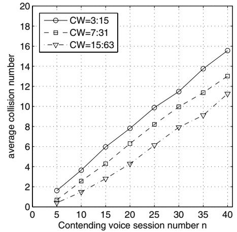
Fig. 5. Average voice collision number (via simulations) in a CP in our scheme.
