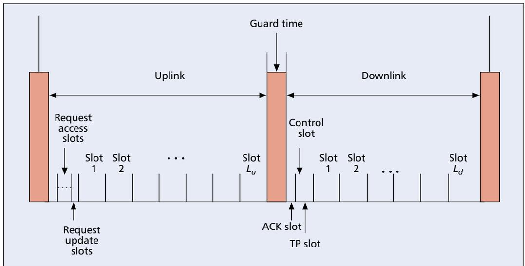
■ Figure 1. Time slots for the uplink and downlink in each frame.
